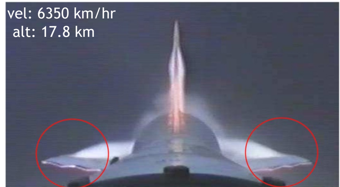
Rear section of SHEFEX-I during decent. Circles indicate control surface LE deformation due to FTSI.
