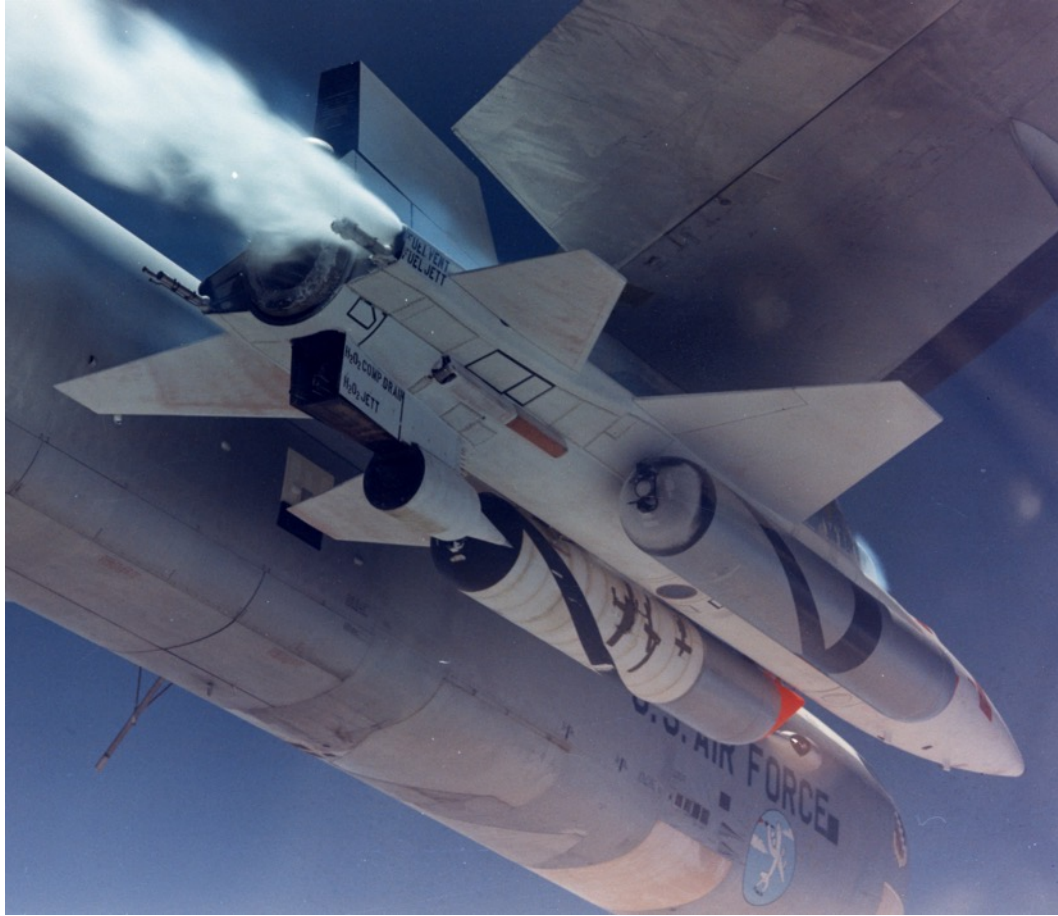
X-15-2 carrying pylon-mounted dummy scramjet Credit: USAF
