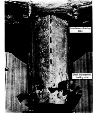
Unanticipated shock-shock interaction caused loss of “engine”, severe damage to pylon (Watts, 1968)
